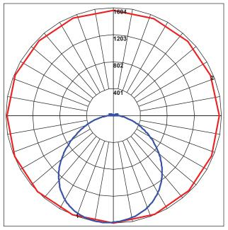
Maximum Candela = 1603.9 Located At Horizontal Angle = 270, Vertical Angle = 6 # 1 - Vertical Plane Through Horizontal Angles (270 - 90) (Through Max. Cd.) # 2 - Horizontal Cone Through Vertical Angle (6) (Through Max. Cd.)
