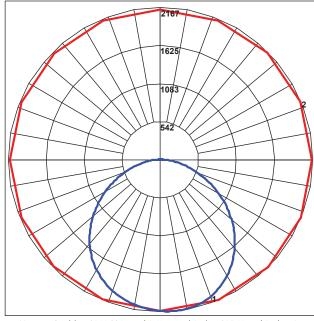
Maximum Candela = 2166.88 Located At Horizontal Angle = 315, Vertical Angle = 4 # 1 - Vertical Plane Through Horizontal Angles (315 - 135) (Through Max. Cd.) # 2 - Horizontal Cone Through Vertical Angle (4) (Through Max. Cd.)
